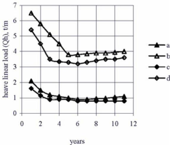
Fig. 3 Variation of heave linear load with time and permeability coefficient (a -  $K_f = 10^{-9} \frac{m}{s}$ ,  $T_{\text{gas}} = -2, -7 \text{ °C}$ ; b -  $K_f = 10^{-10} \frac{m}{s}$ ,  $T_{\text{gas}} = -2, -7 \text{ °C}$ ; c -  $K_f = 10^{-9} \frac{m}{s}$ ,  $T_{\text{gas}} = -2, -2 \text{ °C}$ ; d -  $K_f = 10^{-10} \frac{m}{s}$ ,  $T_{\text{gas}} = -2, -2 \text{ °C}$ ) and with various temperatures of gas in a pipe
