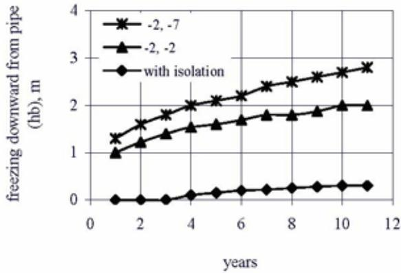
Fig. 2 Change of depth freezing downwards from a chilled gas pipeline under various operating conditions
